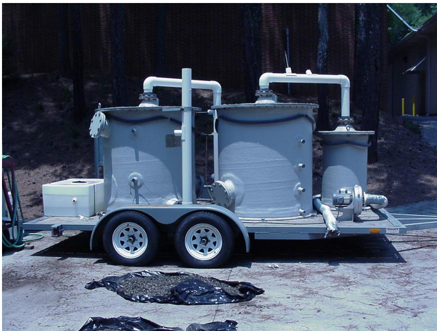
Figure 1. Pilot scale biofilter system configured for in-series flow (humidifier, and Reactors right to left).
