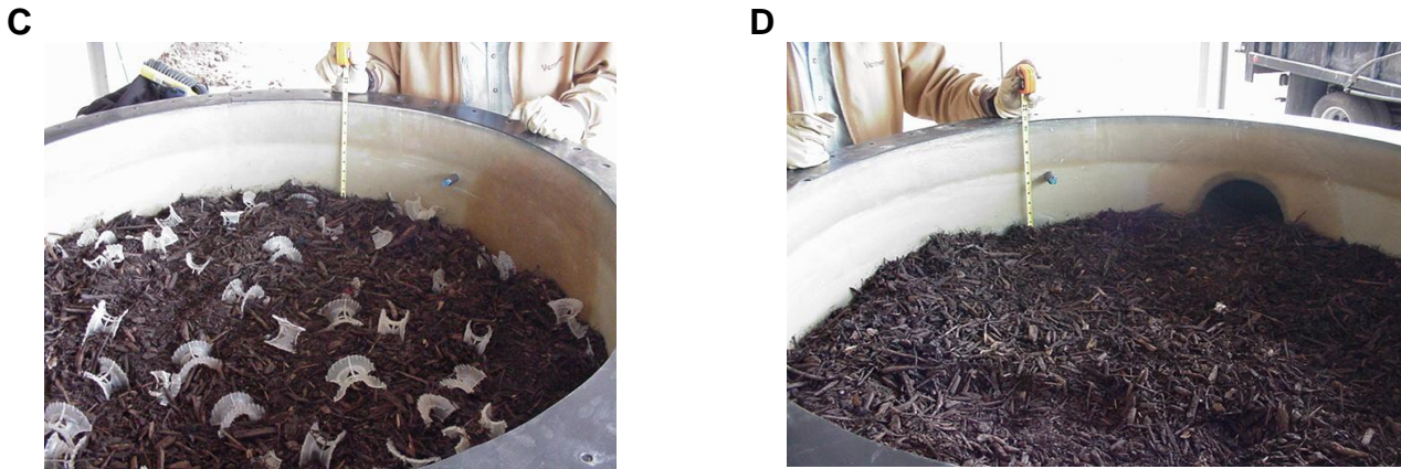
Fig 2: Packing material used in pilot scale biofiltration of ammonia: A – plastic plenum, B and C – compost mixed with inert plastic saddles (Reactor 2) and D – compost only (Reactor 1).
