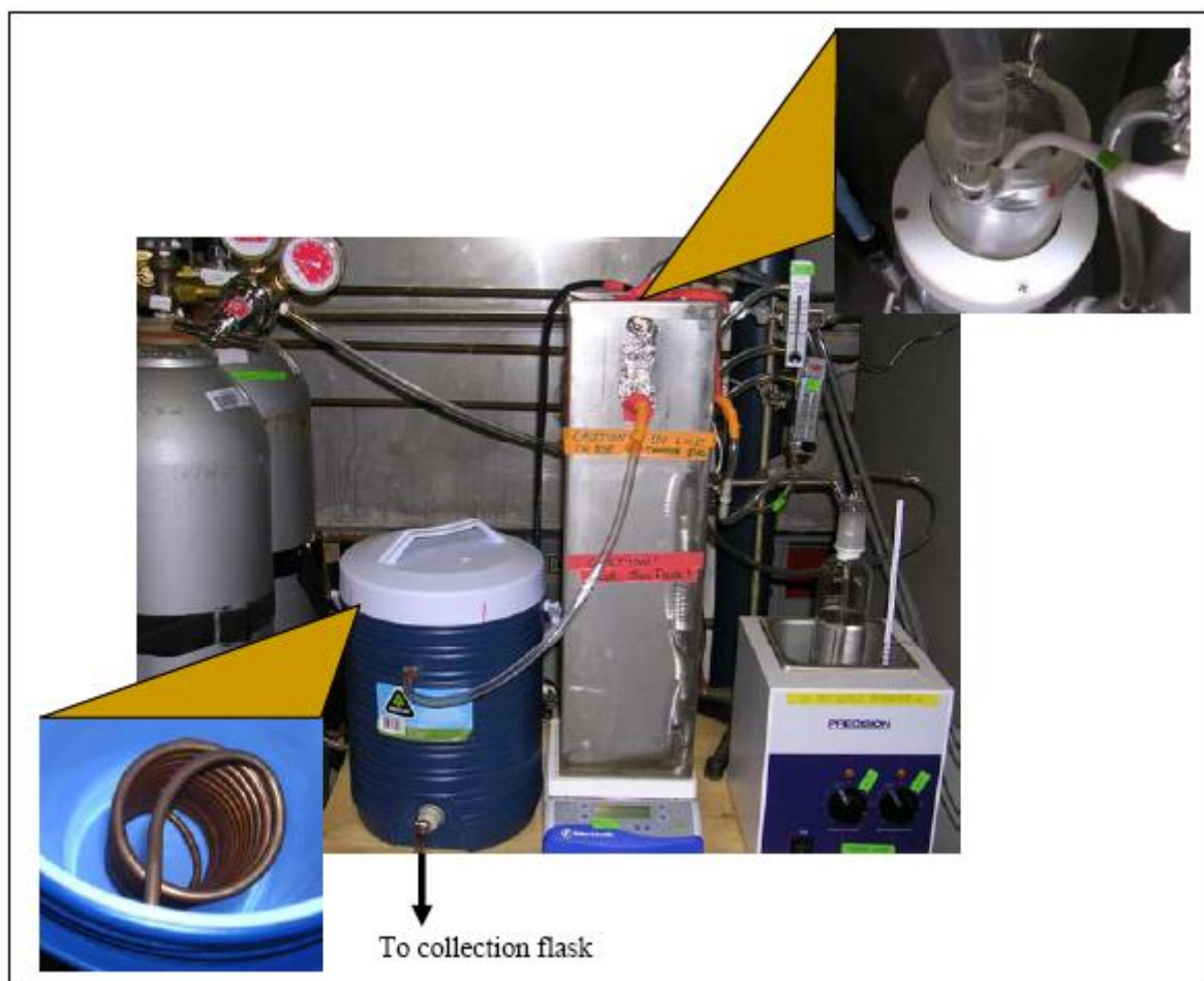
Figure 2: Direct UV/UV-Vis conversion system
