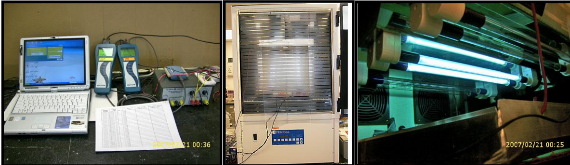
Figure 1. UV exposure data monitoring/acquisition equipment (left). Percival environmental chamber with door open and protective shielding in place (middle). UV 254 emitter (right).
