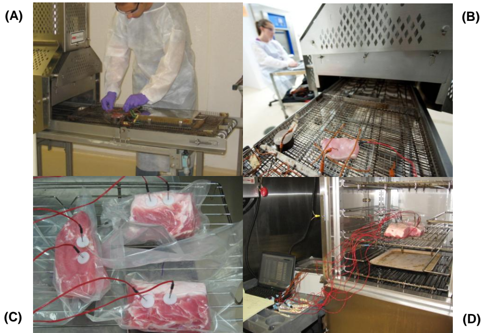
Fig. 2. Inoculated samples being prepared and processed for pilot-scale validation trials. (A) Pork patty being instrumented, (B) Pork chop entering into the impingement oven, (C) Pork roasts prepared for in-bag cooking in convection oven, and (D) Pork roasts in moist-air convection (roasting) oven.
