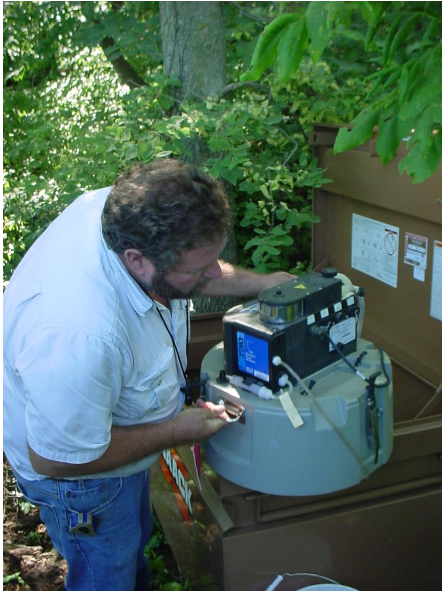
Figure 2: ISCO Portable Sampler being placed in the job-box.
