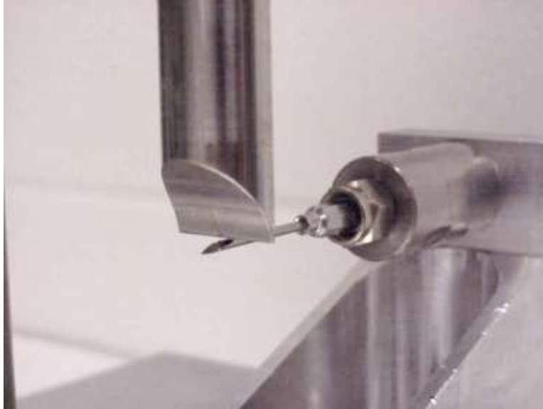
Figure 3. Set-up demonstrating tip-bending testing completed. Maximum load sustained recorded in pounds force (lb f ).
