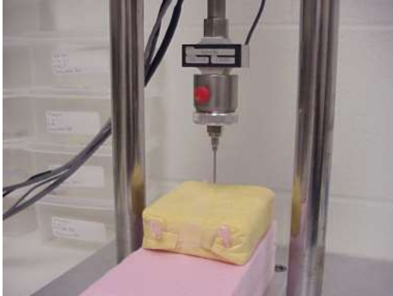
Figure 5. Set-up demonstrating sharpness testing. Maximum puncture force recorded for each injection recorded in pounds force (lb f ).
