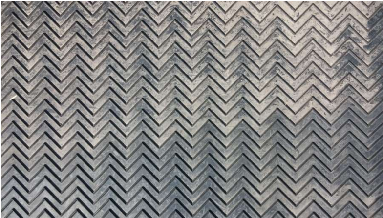
Figure 2. This figure displays the chevron pattern of flooring that comprised the belt of the conveyor. The rise of the texture was approximately 1/8 inch.
