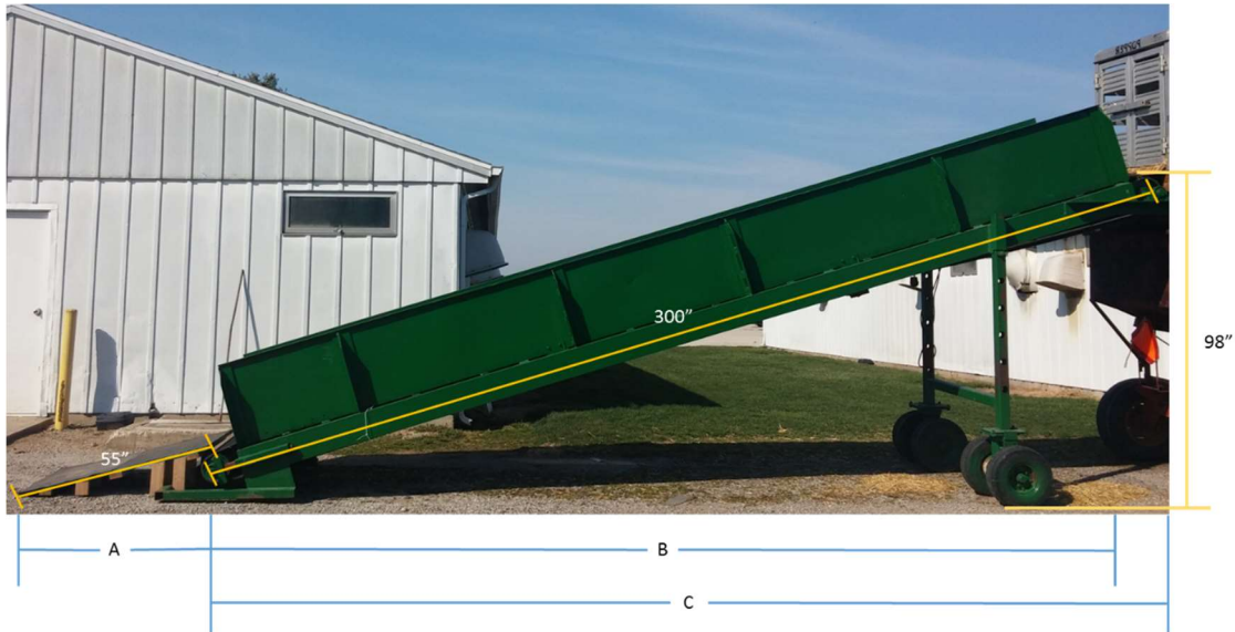
Figure 1. The ramp and conveyor used to load pigs into the simulated trailer. The time pigs spent on the ramp (A), prior to stepping onto the conveyor is denoted as “Botload” in Table 1. The time on the conveyor (B) is denoted as “TrailLat” in Table 1. And the total time to load the pigs starting from when they stepped on the ramp (C) is denoted as “TotTime” in Table 1. The length and height are indicated in the figure.
