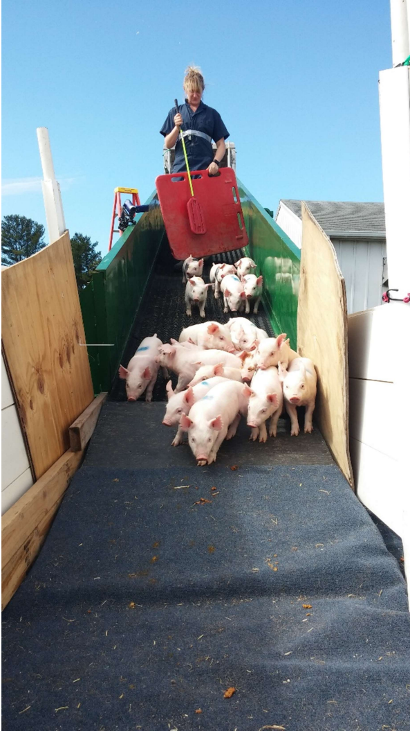
Figure 4. Pigs are being unloaded from the simulated trailer onto a small ramp that connects the conveyor to the ground.
