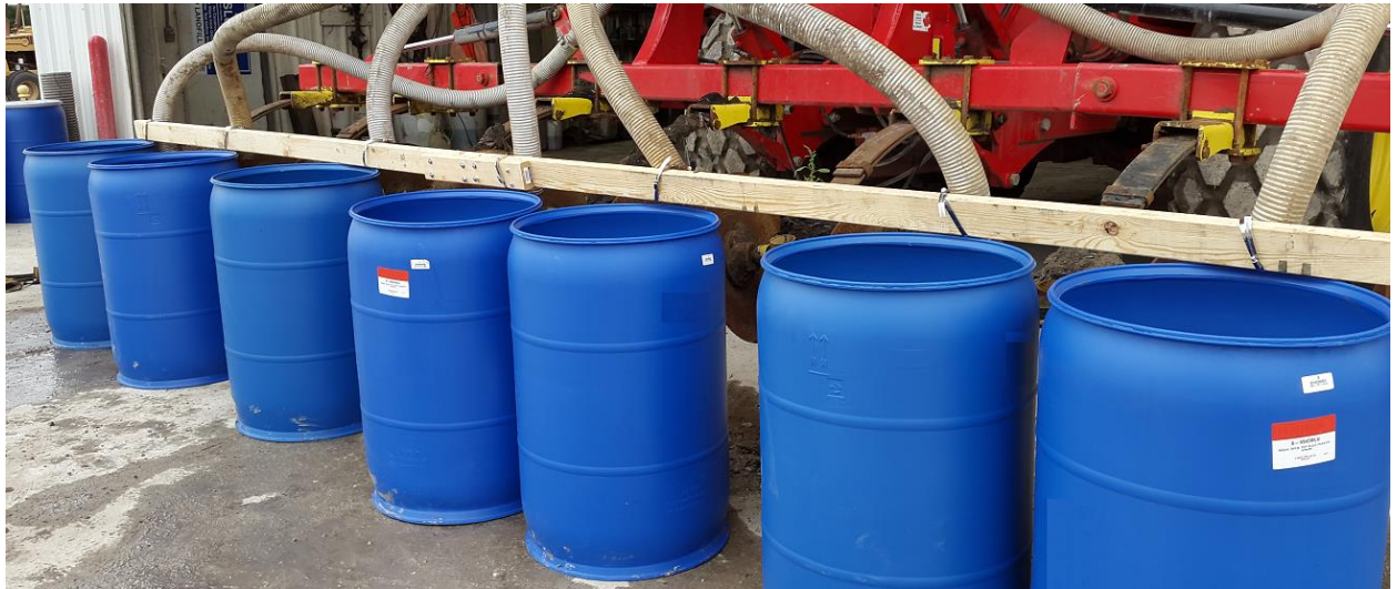
Figure 1: Fifty-five gallon drums arranged underneath the discharge hoses to compare variability across the tool-bar swath.
