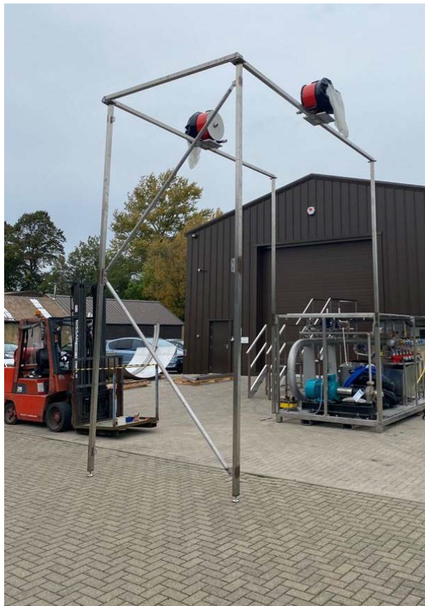
Figure 2 NFDS Foam system with drive through gantry
