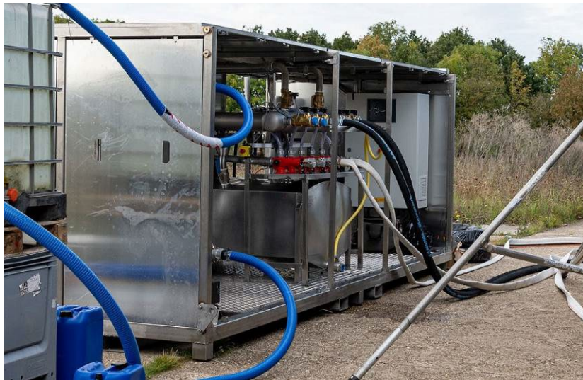
Figure 4. Nitrogen foam system
