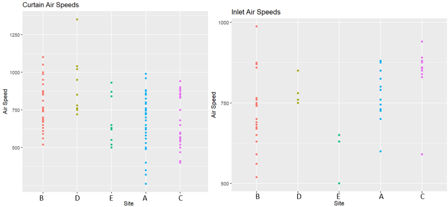
Figure 7. Airspeeds in feet per minute as measured at the curtain (left) and ceiling inlets (right).
