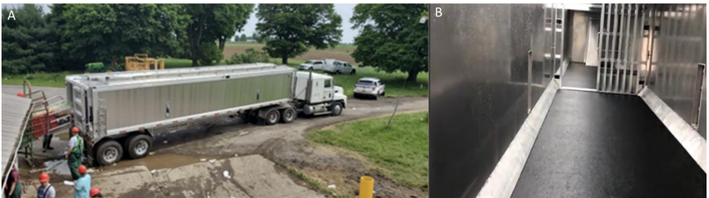
Figure 3. Exterior (A) and interior view (B) of the 84.4-cubic yard modified rendering trailer with a halfwidth/whole gate attached loading ramp and internal center cut-gate for compartmentalization.
