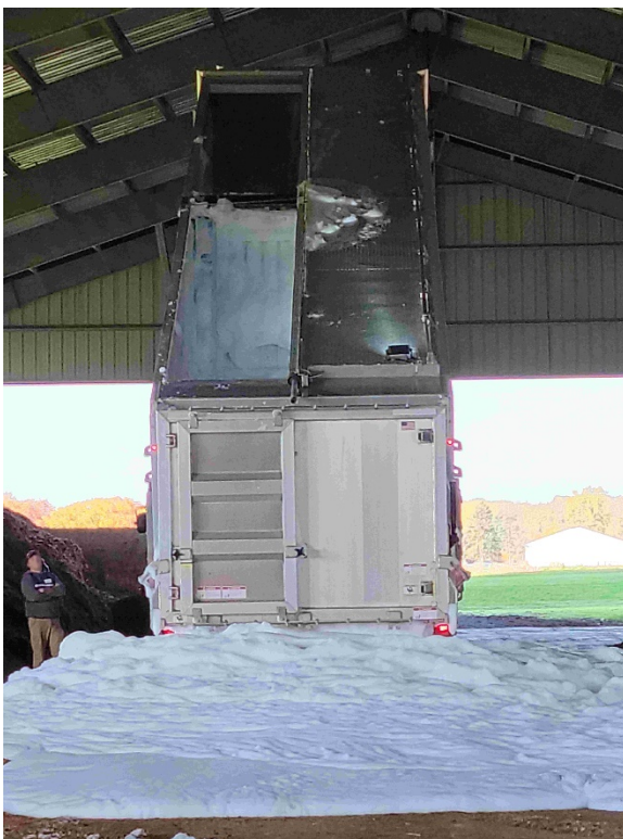
Photo 4. Unloading of water-base foam depopulation trailer inside of Stacking Shed.
