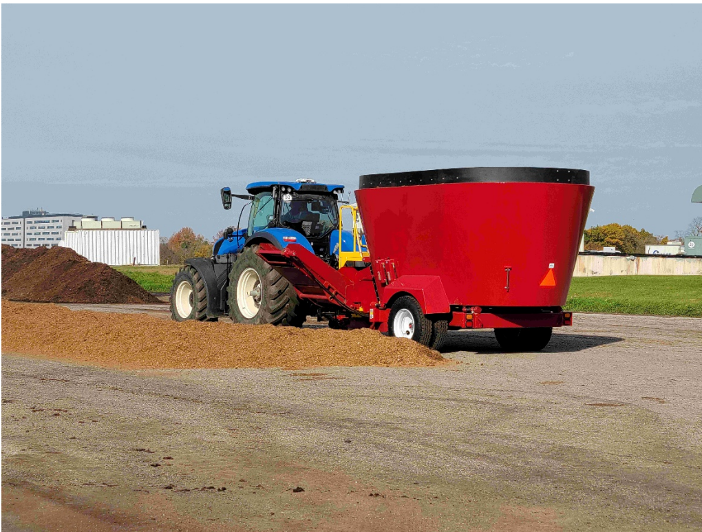
Photo 6. A tub grinder mixer-wagon and tractor that was used to reduce carcasses, prepare compost, and construct the compost windrow.
