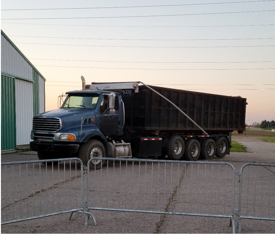
Photo 3. Modified roll-off used for N2 filled foam depopulation of swine.
