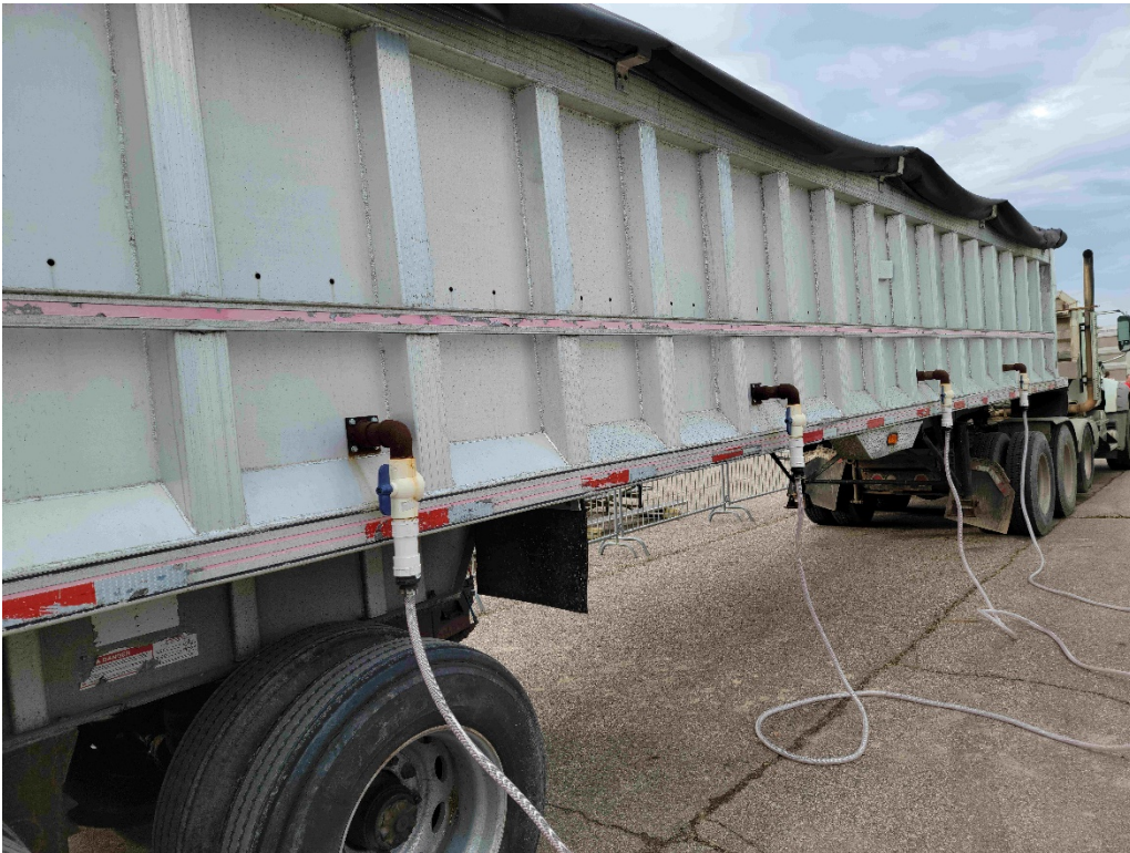
Photo 2. Customized semi-trailer used for CO 2 depopulation of swine.
