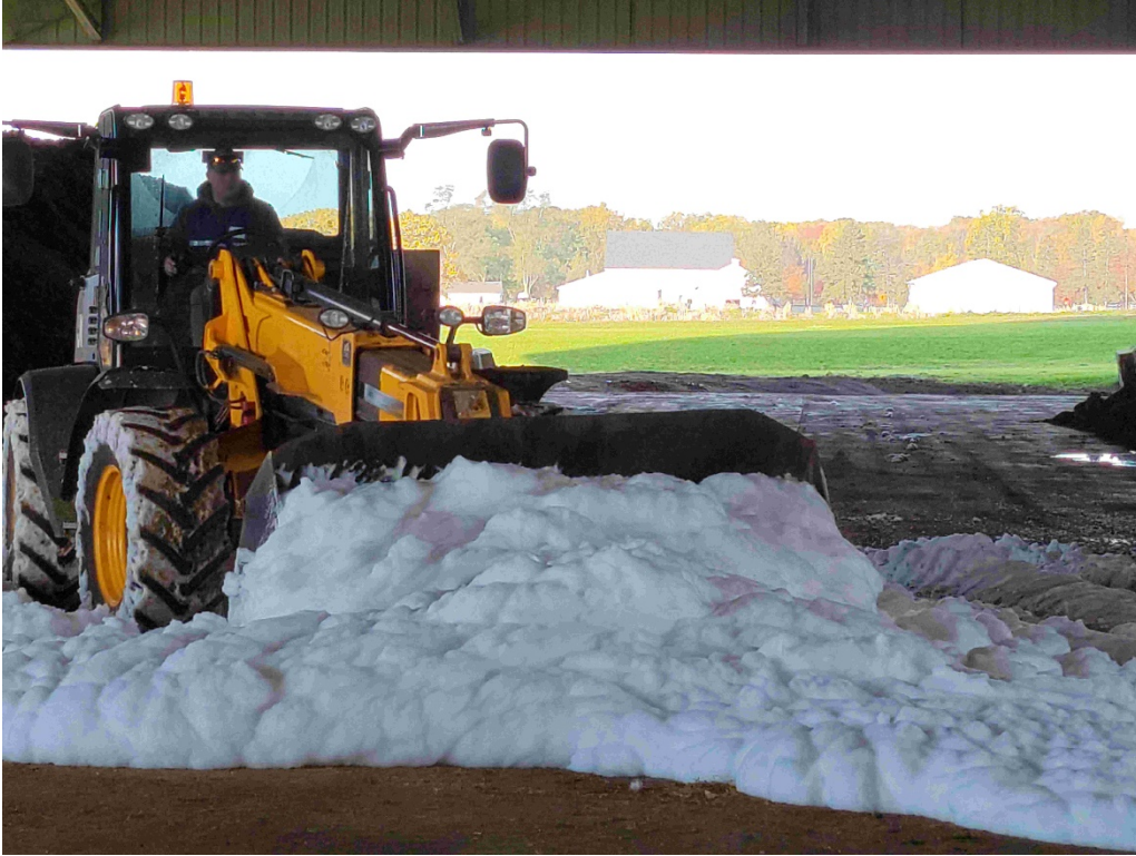
Photo 5. Telehandler loader used to load tub grinder mixer-wagons.
